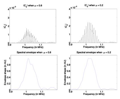
FIG. 2. (Color online) Plots of the fourth-order spectral density,  $|S_4(\omega)|$  (upper panels), and the envelope of the cross-spectrum (lower panels) for the experiment where the degrees of coherence between the fields emitted by the two transducers are 0.8 (left panels) and 0.2 (right panels).
